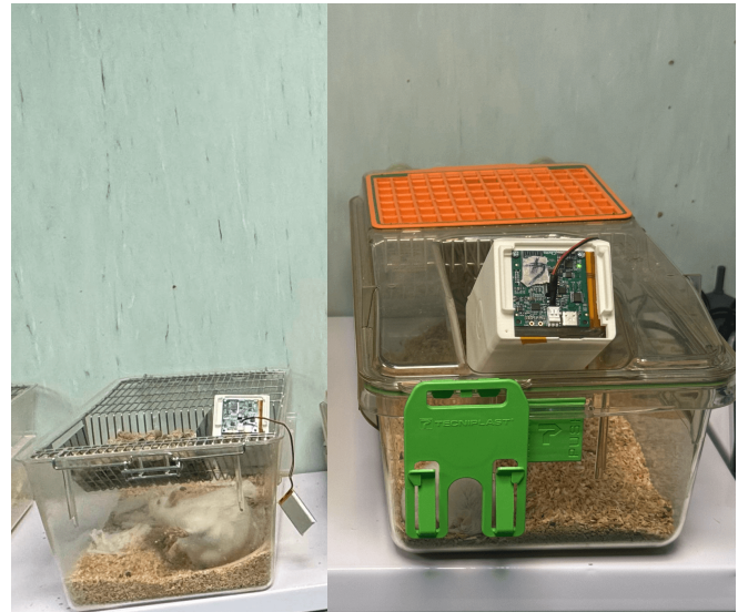
Fig. 4. Shows a real time working prototype system for real time monitoring of liquid intake in lab animals, using sensors based SOC equipped with stainless steel and carbon peek spout of the bottles and data acquisition device mounted on the cage .
