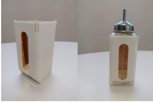
Fig. 2. Shows the custom bottle holder for holding the bottle and Micro-Controller based SOC for monitoring liquid Consumption.
