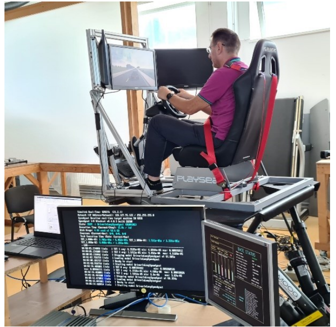
Figure 3. Virtual environment setup, with the MOOG platform and the mounted driving simulator
